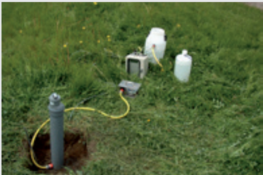
Essai open-end. Source CRR
