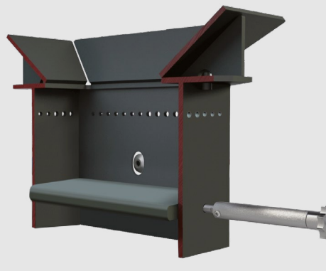
The grate returns to its original position. The stove is ready to turn on again.
